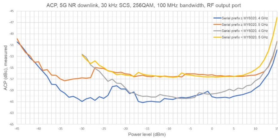
Figure 15. 5G NR downlink ACP vs. output power level at 4 GHz and 5 GHz with 100 MHz bandwidth, 30 kHz SCS, 256 QAM
