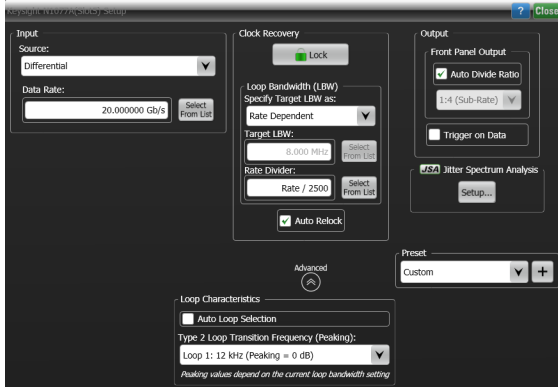
Figure 11. Easily configure the N107x clock recovery data rate, loop bandwidth, and peaking using the N1010A FlexDCA user interface running on an N1000A DCA-X mainframe or standalone PC.
